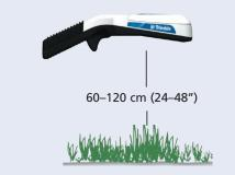
The sensor's field of view is an oval; the field of view widens as the height of the sensor above the ground increases.
