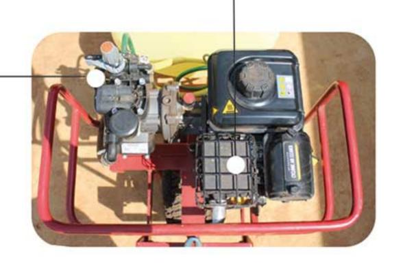
Pump: Comet APS41 3-diaphragm Flow Rate: 40 Litres/ minute | Max. Pressure: 40 Bar
