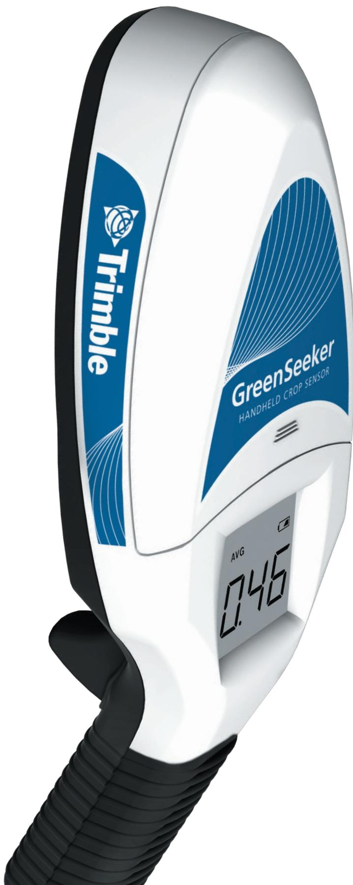
The GreenSeeker handheld crop sensor is an affordable, easy-to-use measurement device that can be used to assess the health—or—vigour of a crop. Readings taken by the GreenSeeker handheld can be used to make non-subjective decisions regarding the amount of fertiliser to be applied to a crop, resulting in a more efficient use of fertiliser—a benefit to both a farmer's bottom line and the environment.
